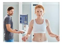
SCANNER AND CAMERA Beams of light are projected to form patterns on the object being measured and are captured digitally. From the information in the images, the software generates a precise 3D model.
